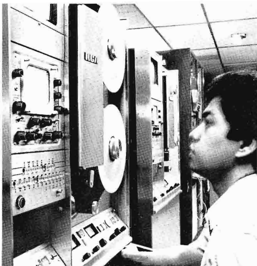
Video taping with one of the four TR-60 machines in the VTR studio.
